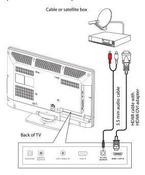
5 Connect a 3.5 mm audio cable (not included) to the PC/DVI AUDIO IN jack on the back of your TV and to the AUDIO OUT jack on the cable or satellite box.
